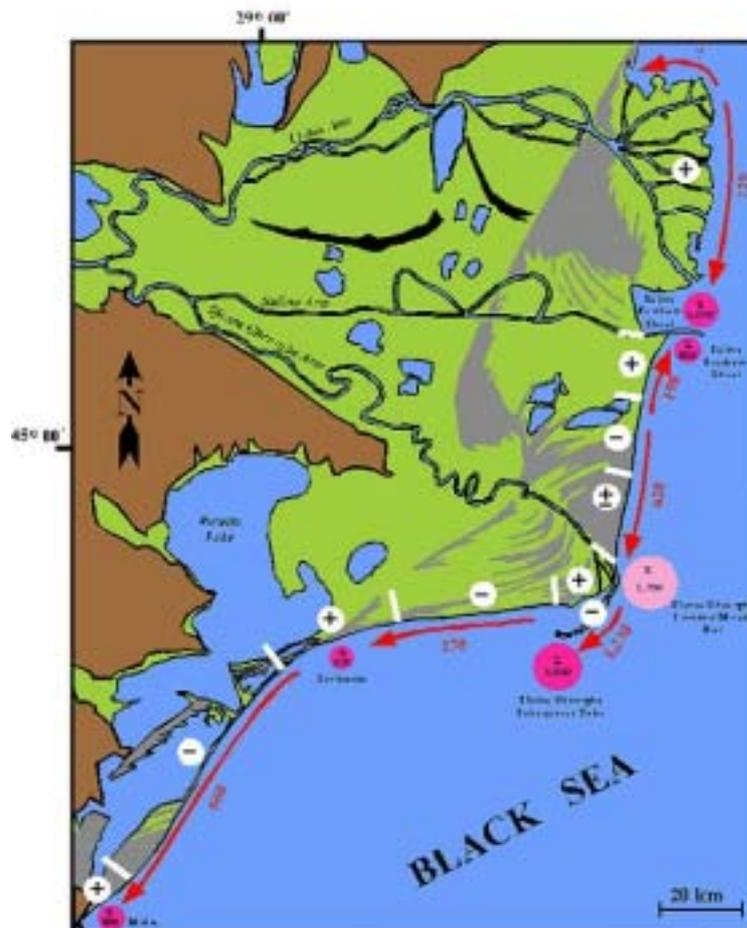
Fig. 6: Longshore sediment transport model for Danube delta coast. Rates and sink volumes are given in 10<sup>3</sup> m<sup>3</sup>/yr.
