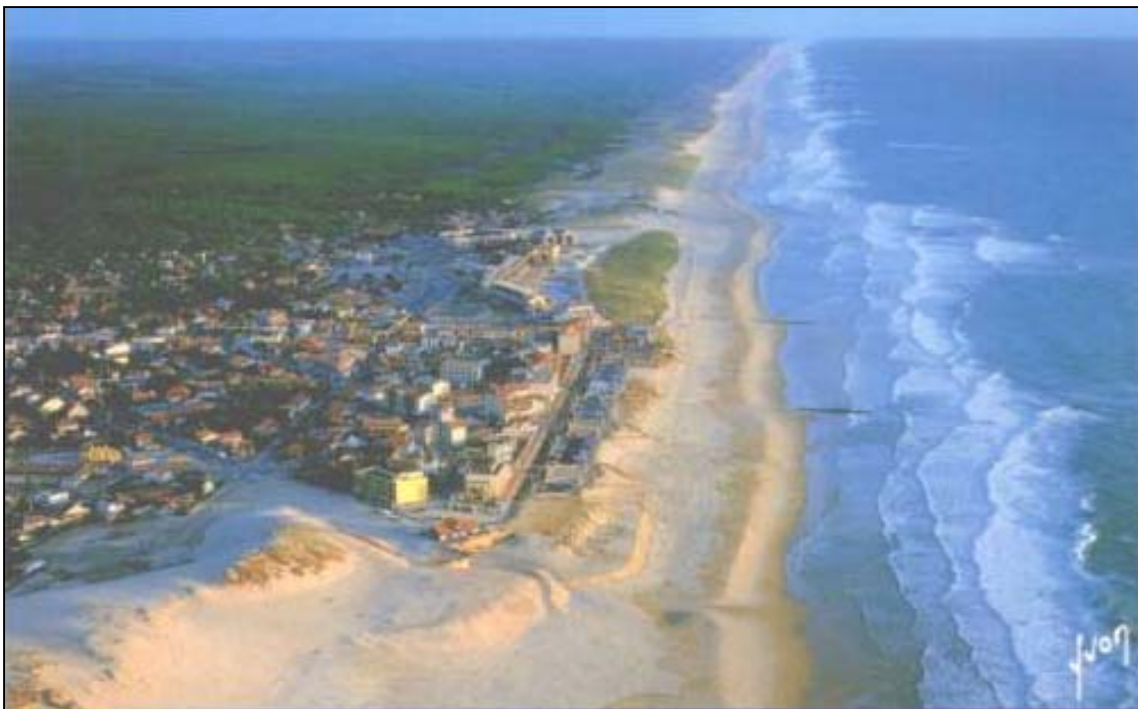
Fig. 6: South view of the Lacanau town. Visible are a few groins constructed to retain sediment of the longshore drift in front of the town.
