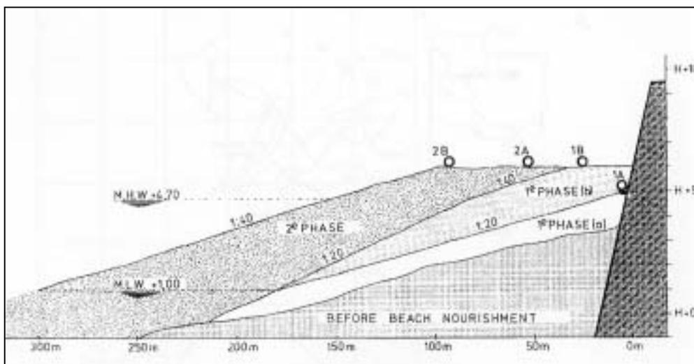
Fig. 7: Cross section of nourished beach at Knokke-Heist.
