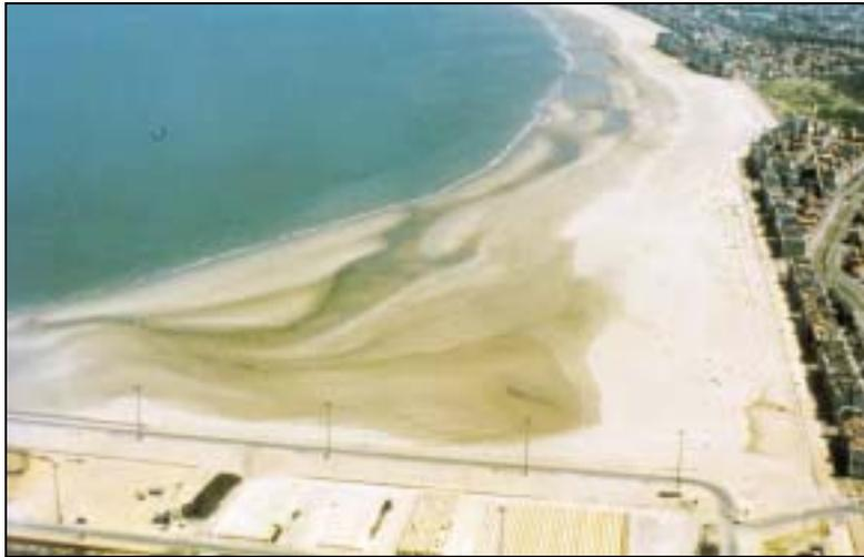
*Fig. 9: Nourishment directly downstream of harbour breakwater.*
