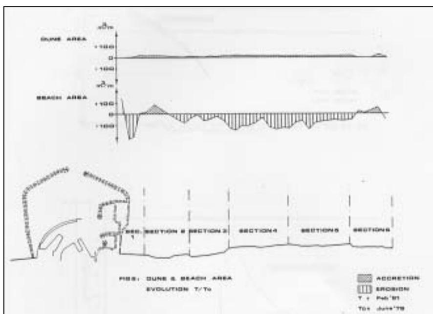
Fig. 8: Erosion and accretion after the first nourishment.
