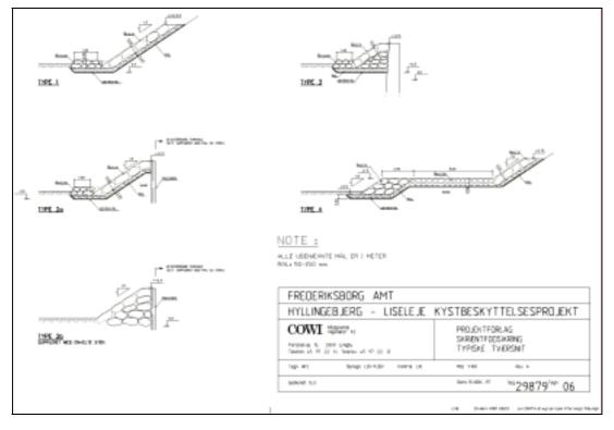
Fig. 9: Different types of slope protection applied at Hyllingebjerg-Liseleje coast.
