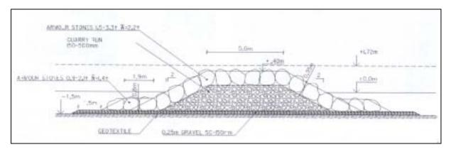
Fig. 5: Typical cross section of a breakwater.
